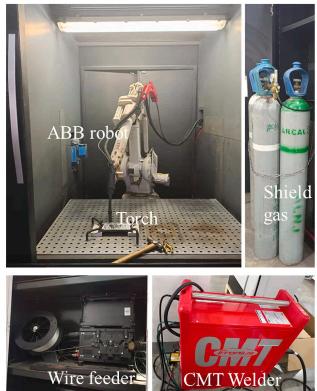
Fig. 1. Main components of CMT-WAAM system.
